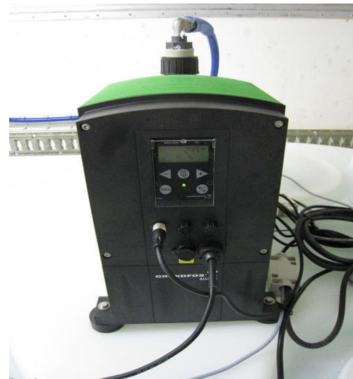
The dosing pump
